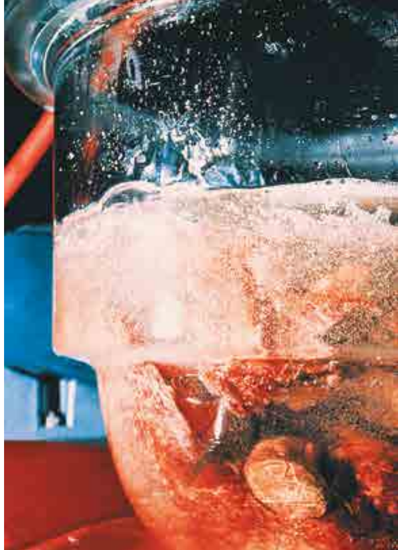
Forced impregnation: Under vacuum conditions, acetone bubbles out of the specimen and is continuously removed, creating negative pressure inside the specimen and allowing the polymer solution to diffuse into it.
