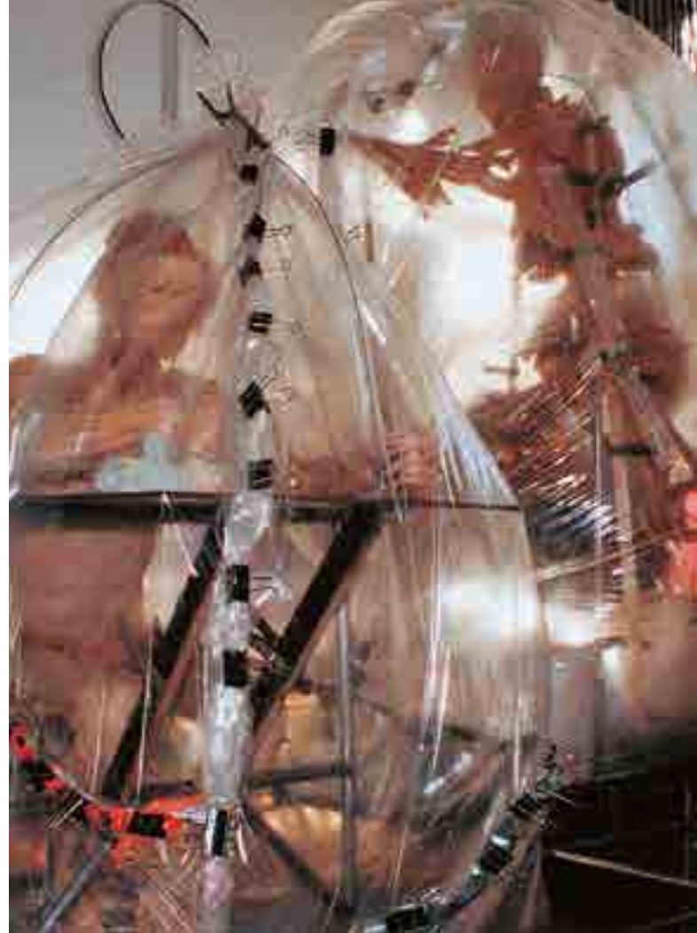
Silicone-impregnated specimens are cured using a special gas in an airtight chamber.
